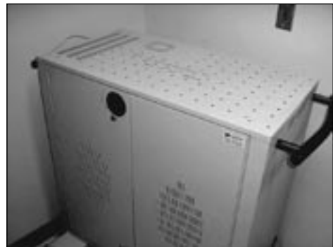
Proposed computer cart stores and recharges up to 20 laptop computers with wireless internet accessibility. The cart is mobile and can be shared between classrooms.
